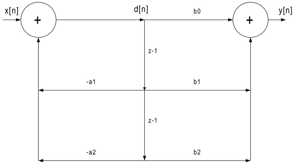
The difference equations used for implementation of the direct form II structure shown in Figure 1:
