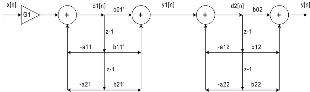
In Figure 3, the scale factor of section 2,  $G_2$ , is used to scale the  $b_i$  coefficients of section 1 as follows:
