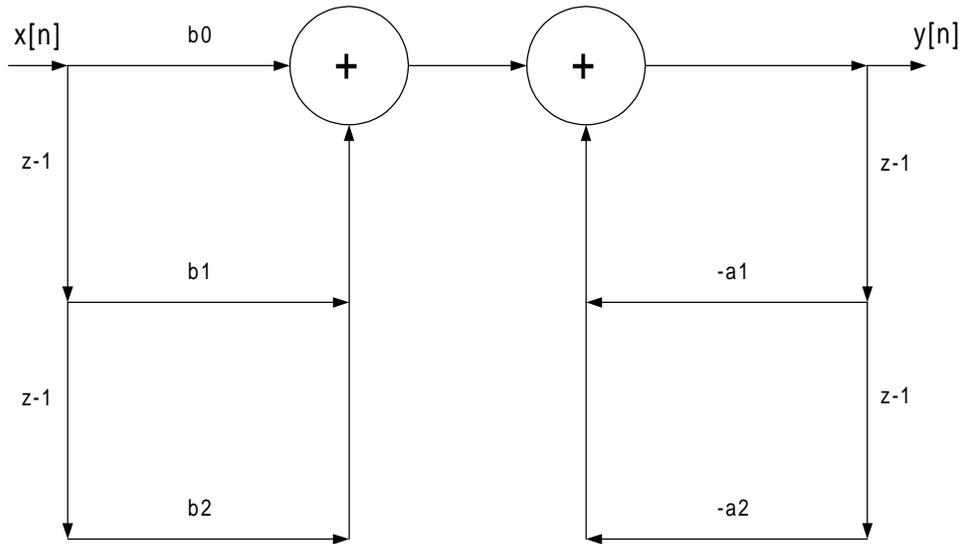
The difference equation used for implementation of the direct form I structure shown in Figure 2 is:
