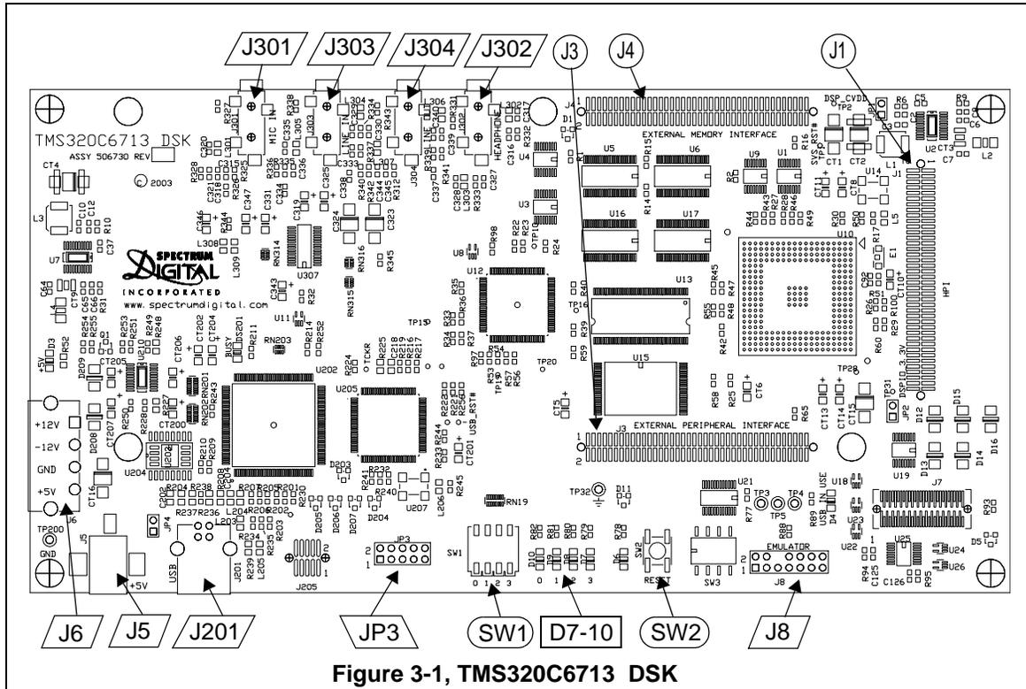
Figure 3-1, TMS320C6713 DSK
