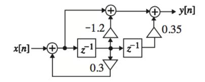
(d) A partial-fraction expansion of H(z) in  $z^{-1}$  using residuez is given by  $H(z) = 0.1111z^{-1} - 1.1667 + \frac{0.8889}{1 - 0.3z^{-1}}$  whose realization yields the Parallel Form I structure shown below.
