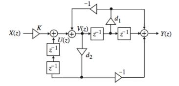
$U(z) = KX(z) + d_2 z^{-1}V(z), V(z) = U(z) - d_1 z^{-1}V(z), Y(z) = d_1 z^{-1}V(z) - z^{-2}V(z) - d_1 V(z).$ Eliminating the internal variables we arrive at
