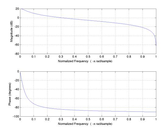
Note the lowpass nature of this transfer function, which is what we would expect with a zero at z = -1 and a pole at z = 0.9. Also note that Matlab is only plotting the magnitude and phase on  $\omega \in [0, \pi]$ , which is sufficient to understand the whole spectrum due to the symmetry and periodicity properties of the DTFT of a real sequence.
