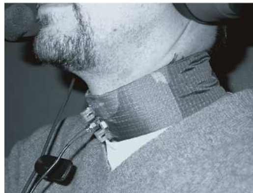
Figure 4. Photograph of the placement of the single-mode TERC sensor.
