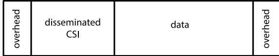
Fig. 2: Example fixed-length packet showing overhead, data, and CSI dissemination. The CSI dissemination consists of M channel estimates and each channel estimate has a length of one word. The data and overhead consists of D words. The total packet length is P = D + M words.
