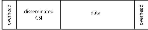
Fig. 1. Example fixed-length packet showing overhead, data, and CSI dissemination. The CSI dissemination consists of M \in \{1, \dots, N - 1\} channel estimates and each channel estimate has a length of one word. The data and overhead consists of D words. The total packet length is P = M + D words.
