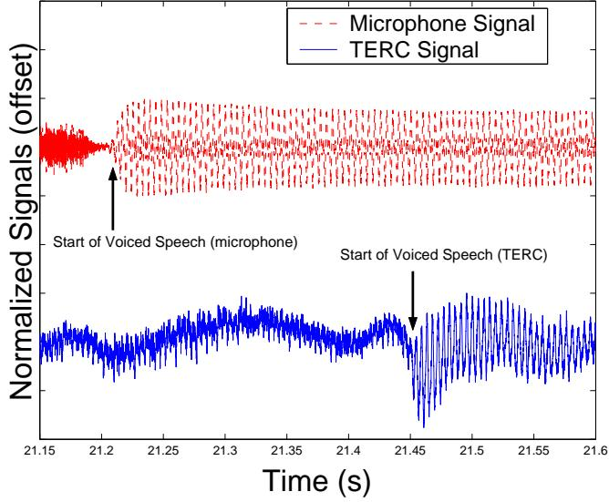
Figure 5.3: Delay between the TERC and microphone signals.
