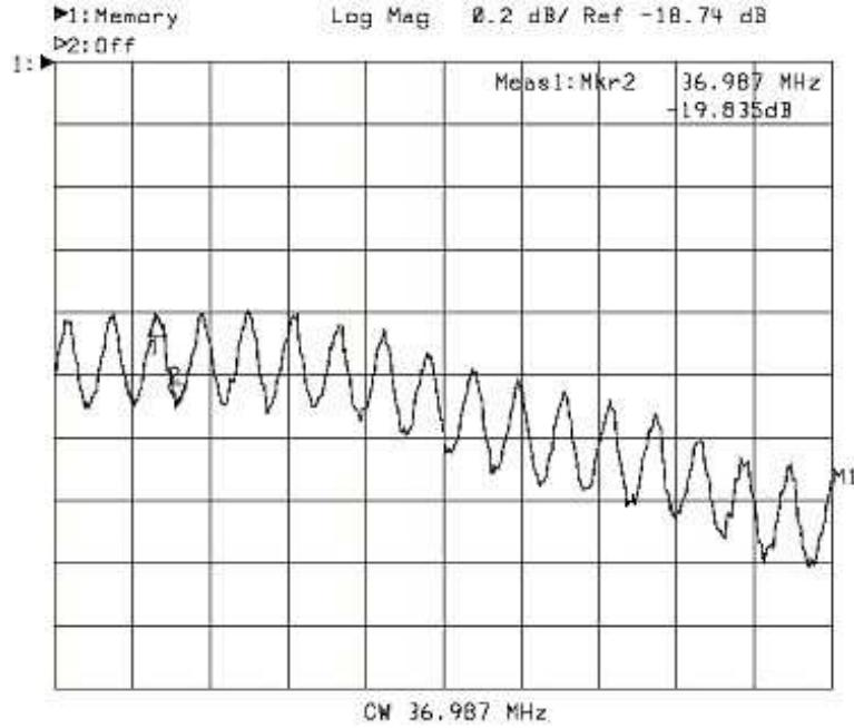
Figure 3.4: Baseband glottal signal from TERC sensor during voiced speech as seen on Network Analyzer [Pel04].
