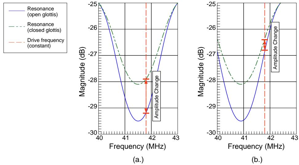
Figure 4.5: Concept behind using an AM system (a) and the effect of resonance shifts on the system (b).
