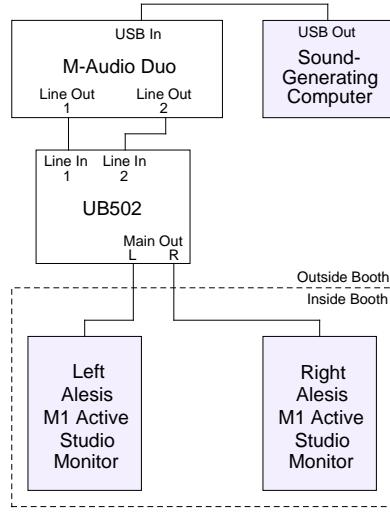
Figure 4.3: Environmental Noise Production System Setup.
