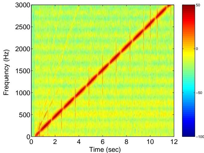
Figure 5.6: Spectrogram of linear frequency sweep with "spatial" setting on.
