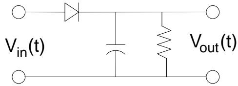
Figure 3.6: Diode/capacitor envelope detector circuit.
