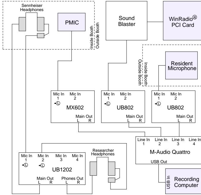
Figure 4.4: Recording System Setup.
