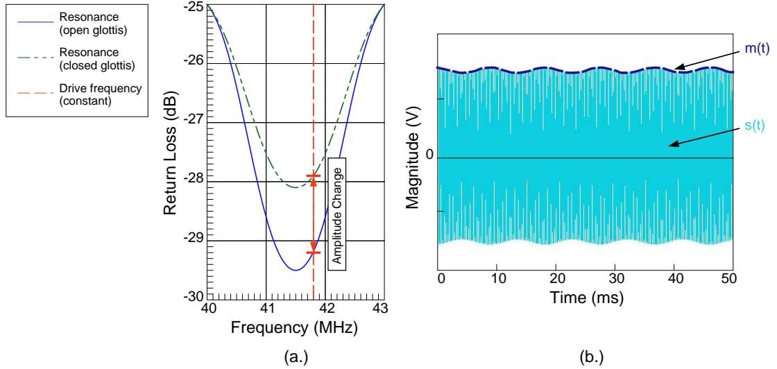
Figure 3.3: The changes to the resonance caused by the glottal cycle (a) result in an amplitude modulated voltage waveform (b).
