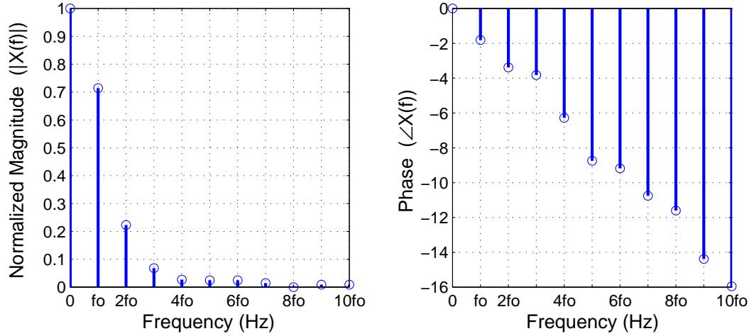
Figure 2.3: Approximate frequency response of the glottal waveform.
