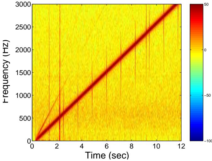
Figure 5.7: Spectrogram of linear frequency sweep with “spatial” setting off.
