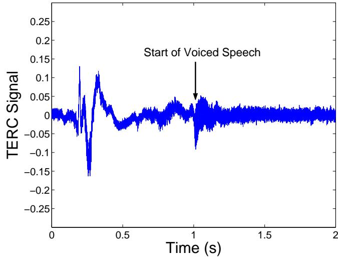
Figure 5.2: Low frequency signal content prior to voiced speech.
