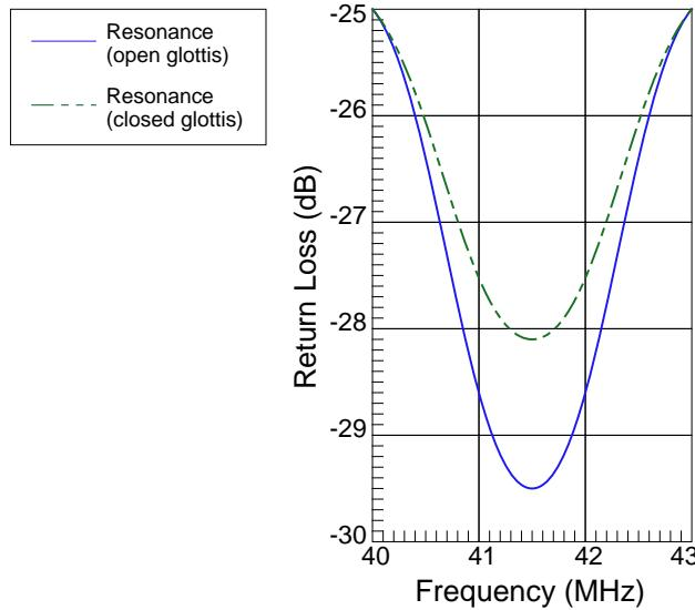
Figure 3.2: Theoretical resonance shift due to glottal state changes.
