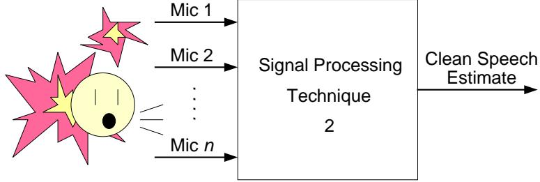
Figure 1.2: Signal processing techniques using multiple microphones in an array.
