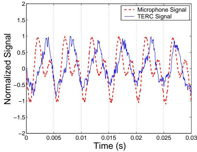
Figure 5.1: Time domain comparison between microphone and TERC signals.
