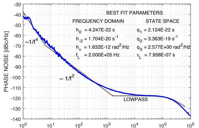
Fig. 9. Measured phase noise for oscillator CS8 with 3-state model fit.
