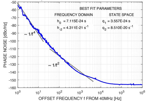
Fig. 6. Measured phase noise for oscillator CS4 with 2-state model fit.
