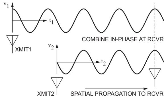
Fig. 1. Conceptual beamforming.
