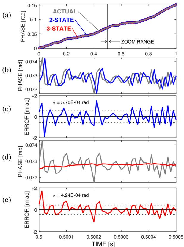
Fig. 10. Prediction for oscillator CS8 with 2- and 3-state model fits.
