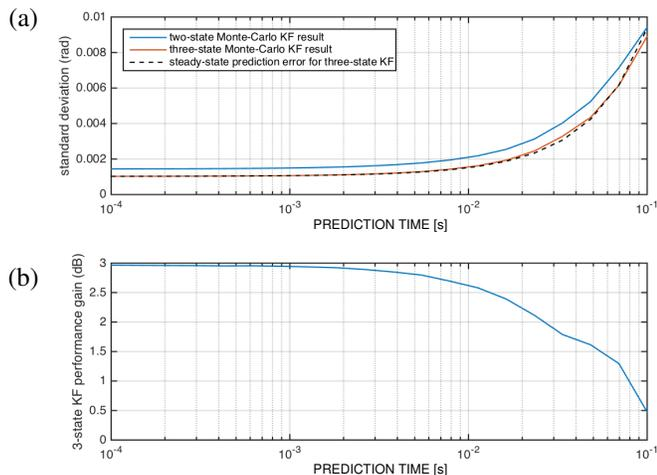
Fig. 11. Relative performance, 2-state vs. 3-state model fit.
