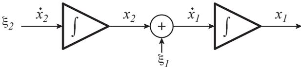
Fig. 5. 2-state clock noise model
