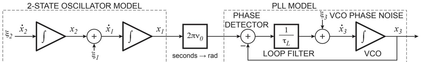
Fig. 7. Three-state model for phase noise of source with PLL synthesizer
