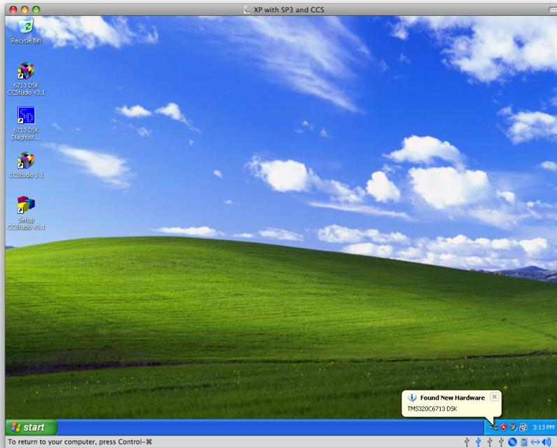
Plug the USB cable from the DSK into the computer. Power up the DSK. The computer should detect new hardware via the “Found new hardware” popup.
