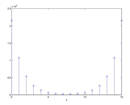
Figure 1: Total quantization error in product as a function of k for the example with  $M_x = 11$ ,  $M_y = 13$ ,  $N_x = N_y = N_z = 16$  and  $M_z = 9$ .
