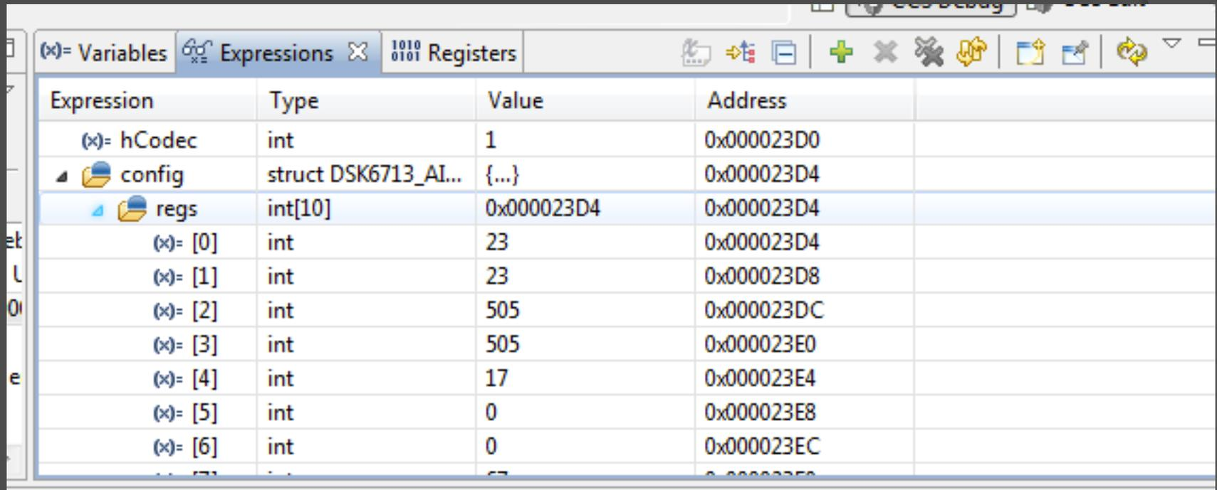
The screenshot shows a debugger window with the 'Expressions' tab selected. The window displays a list of global variables and their values. The variables are organized into a tree structure under the 'config' and 'regs' folders. The 'regs' folder is expanded, showing an array of 10 integers. The values for the first seven elements of the array are 23, 23, 505, 505, 17, 0, and 0.
