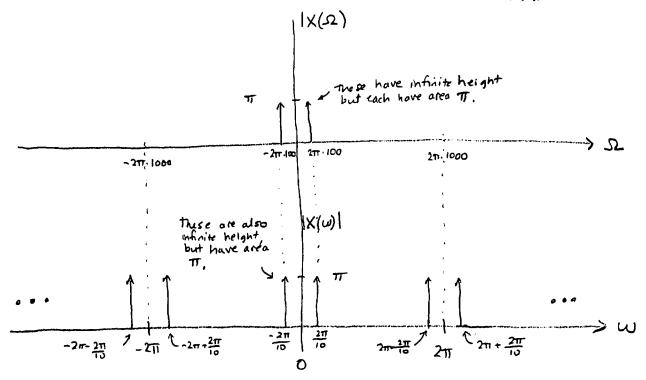
$$\chi(t) = \frac{1}{2}e^{j\Omega_{0}t} + \frac{1}{2}e^{-j\Omega_{0}t} \stackrel{CTFT}{\longleftarrow} \chi(\Omega) = \pi \delta(\Omega-\Omega_{0}) + \pi \delta(\Omega_{0}+\Omega_{0})$$
