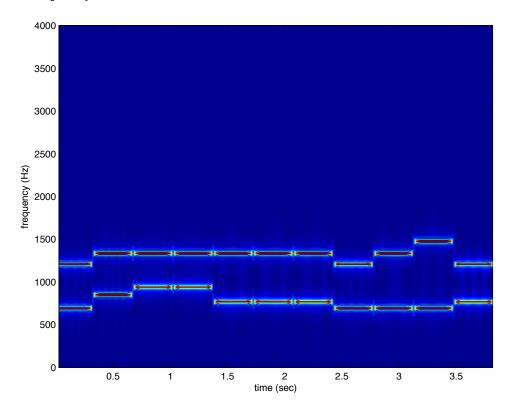
Zooming in on the figure suggests the following approximate frequency pairs and corresponding DTMF digits:
