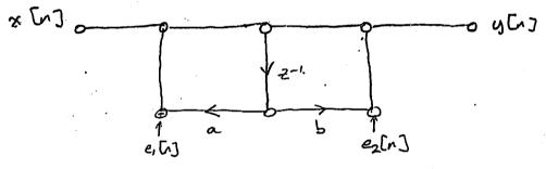
e\_[n] is directly connected to the output  $e_1[n]$  propagater through  $H(2) = \frac{1+b2^{-1}}{1-a2^{-1}} = \frac{72+b}{2-a} = 1+\frac{a+b}{2-a}$
