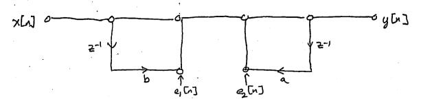
Note that e, [1] and e, [1] both propagate through just the first-order system G(2) = 1 - 1 - 2 - 1
