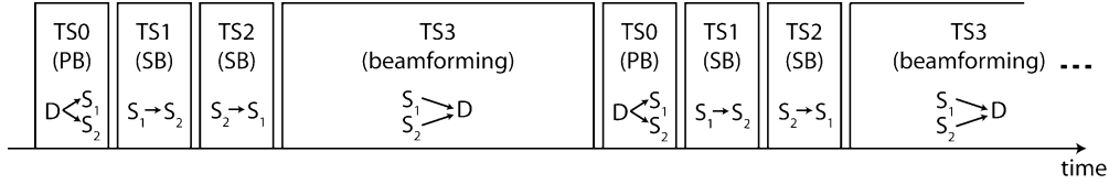
Fig. 2. Summary of the two-source time-slotted round-trip carrier synchronization protocol where PB and SB denote primary and secondary beacon synchronization timeslots, respectively.
