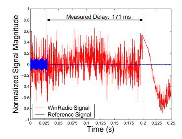
Figure 5.4: Delay through the WinRadio package after input signal turned off.
