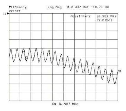
Figure 3.4: Baseband glottal signal from TERC sensor during voiced speech as seen on Network Analyzer [Pel04].
