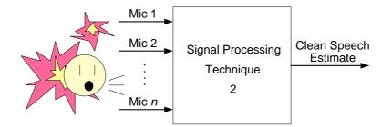
Figure 1.2: Signal processing techniques using multiple microphones in an array. tibility to environmental noise is still high when using only traditional acoustic microphones. Rather than assuming that the input to the system has to be an array of acoustic microphones, the model in Figure 1.2 can be amended to include more generic "sensor" inputs:
