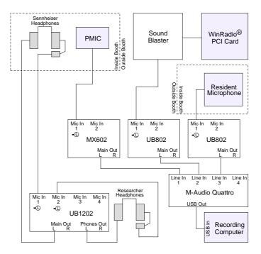
Figure 4.4: Recording System Setup.
