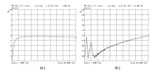
Figure 3.5: Forward transmission on Network Analyzer with circulator port 2 open (a.) and terminated (b.).
