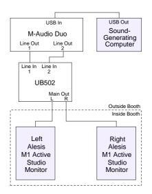
Figure 4.3: Environmental Noise Production System Setup.
