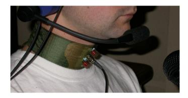
Figure 4.2: Physical location of the TERC sensor on a human subject's neck.
