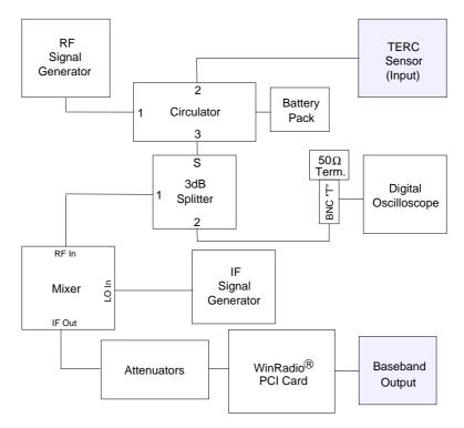
Figure 3.7: Signal Acquisition Setup for the TERC Sensor.
