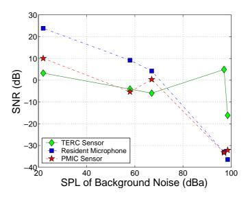
Figure 5.10: SNR versus SPL measurements for three sensors.
