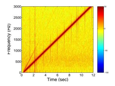
Figure 5.7: Spectrogram of linear frequency sweep with "spatial" setting off. dips in the PSD in Figure 5.8 at the same locations as the nulls from the spectrogram in Figure 5.5 do not appear in the PSD in Figure 5.9 where the "spatial" setting was turned off.
