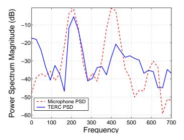
Figure 5.11: Comparison of PSD for microphone and TERC sensors.
