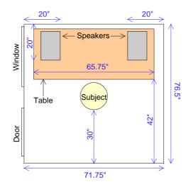
Figure 4.1: Interior layout of the sound booth during testing.
