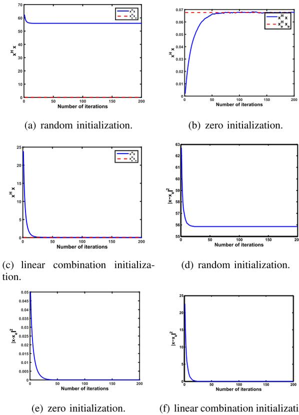
Fig. 5. In (a,b,c), blue line represents the total transmit power, red dashed line represents the power corresponding to power efficient solution. (d,e,f) represent the deviation of transmit weights from optimal weights under the JBNF algorithm.
