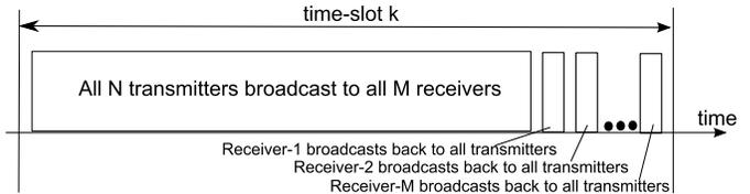
Fig. 2. Description of transmission in time-slot  $k$ .
