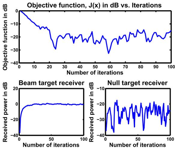
Fig. 8. JBNF algorithm with a time-varying channel.
