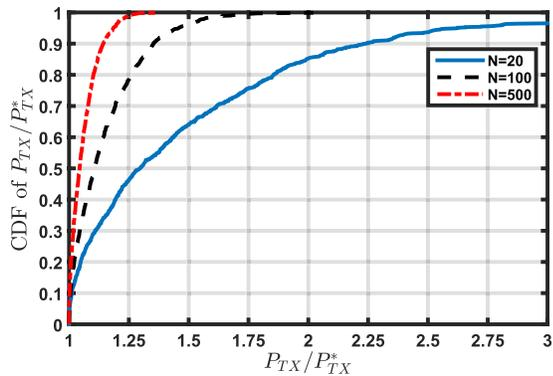
Fig. 7. Cumulative Distribution Function of transmit power corresponding to power efficient solution.
