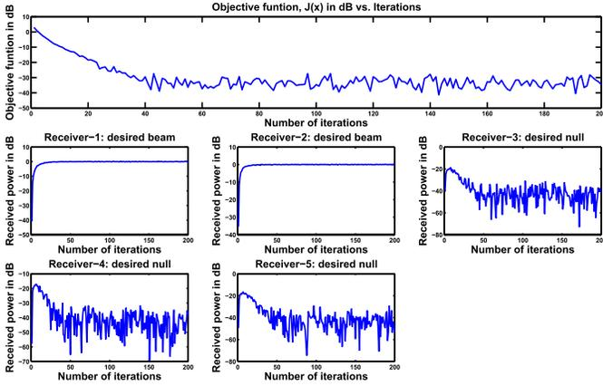
Fig. 4. Convergence of JBNF algorithm with initialization of transmit weights as zeros.
