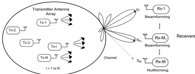
Fig. 1. Problem of joint beam and null-forming using a distributed array.
